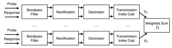
FIGURE 1: Block diagram for STI calculation.
